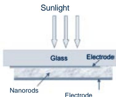
Schematic diagram of a hybrid "plastic" solar cell with a nanorod/polymer layer sandwiched between two electrodes.
