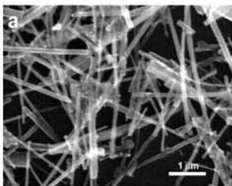
*These nanowires of potassium niobate act as miniature lasers that are small enough to be placed inside human cells, where they can act as both mechanical and optical probes.*
